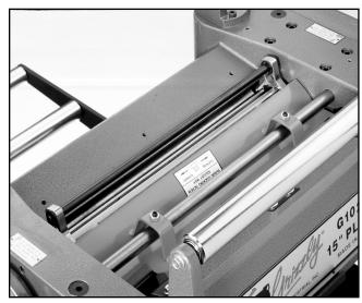
Figure 15. Cover Removed, Jig on cutterhead
